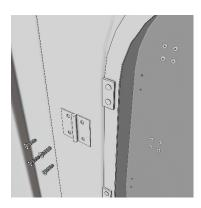
**DO NOT** over tighten hinges to the plexiglass; this can cause the window to crack. Tighten nuts by hand or with a socket. **DO NOT** use Loctite.
