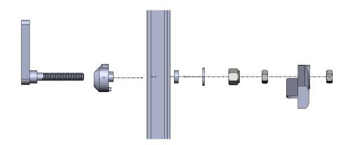
Step 5: Slide the Spacer then the washer onto the threaded stud.
