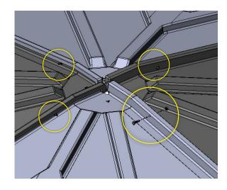
+ When you are bolting the middle hole, you will see two different holes in the metal support bracket. Bolt through the hole that fits best.
