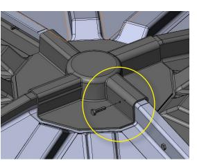
Step 8: You now have a completed 6-Panel Roof. Place roof on top of your constructed wall panels. Be sure the section of roof above the door is flat and does not have a rain guard in the middle.
